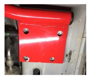
**Step 3.** Remove the brace, and use a 7/16" bit to drill each of the 8 holes.
