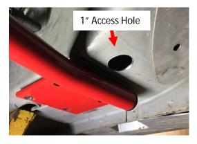
**Step 5.** Reinstall the brace using the two trailing arm nuts (using the golden slotted spacers like in step 1), then attach the 4 frame rail bolts by inserting the nuts into the frame rails and holding them with your finger while you tighten. Eventually the nuts will spin and lock into place against the inside of the frame rail.
