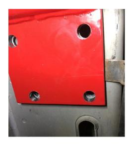
**Step 4.** Use a step bit to drill a 1" access hole outside the mark you made in step 2 for the end of the tube. This hole is where you will insert two of the nuts into the frame rail once the brace is installed. Be sure to drill the hole on the correct side of the line, towards the rear of the car! The closer this hole is to the bar, the easier it will be to hold the nuts in place in later steps!
